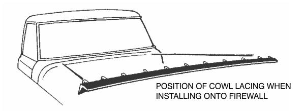
2. Making sure that the horizontal flap of the cowl lacing is facing upward, Install the cowl lacing by snapping the retaining clips into the appropriate holes on the firewall.
