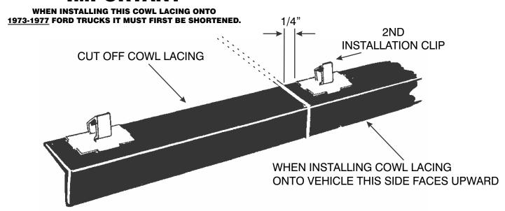
When installing this cowl lacing onto 1973-1977 model trucks, the cowl lacing must be cut shorter in order for the snap-in clips to properly align with the holes on the firewall.
