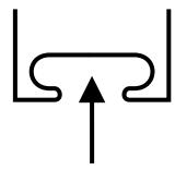
Remove all traces of the old weatherstripping. Clean the swing-out track thouroughly.
