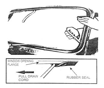
**5.** Position the glass assembly in the opening from the outside and have a helper apply pressure to the outside of the glass. From the inside, begin pulling the draw cord. This procedure allows the rubber seal to be pulled over the window opening flange area. Alternate from side to side when pulling the cord to keep the installation even. The draw cord operation will be completed at bottom center of the windshield. Pull the cord completely out of the rubber seal.
