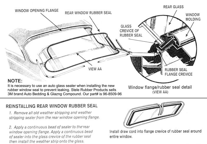
3. Insert the window moldings into the rubber seal before installing the window into the car.
