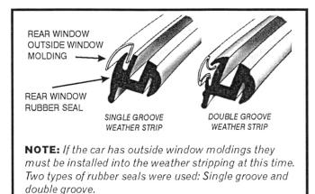
**4.** Reinstall rubber seal onto glass.
