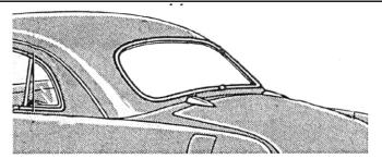
**Installing rear window rubber seal 1.** *Remove all old weather stripping and weather stripping sealer from the rear window opening flange. Clean the flange area thoroughly.*
