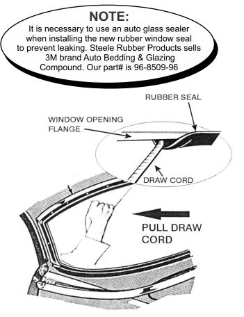
**6.** Position the glass assembly in the opening from the outside and have a helper apply pressure to the outside of the glass. From the inside, begin pulling the draw cord. This procedure allows the weather stripping to be pulled over the flange area. Alternate from side to side when pulling the cord to keep the installation even.
