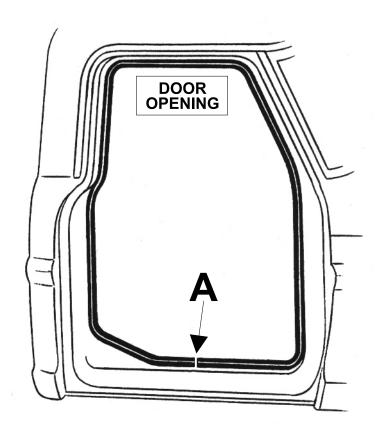
With the door rubber (pressed to the body of the cab - no glue yet) Start inserting at the bottom center (Point A) and go back towards the lock pillar. Continue up the lock pillar to the top, across the top towards the front, down the windshield pillar & hinge pillar finishing at Point A. Trim off extra rubber and begin gluing the rubber seal to the body.
