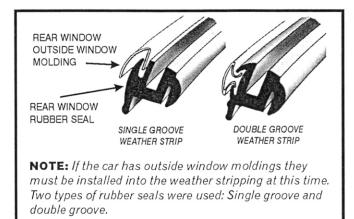
4. Reinstall rubber seal onto glass.
