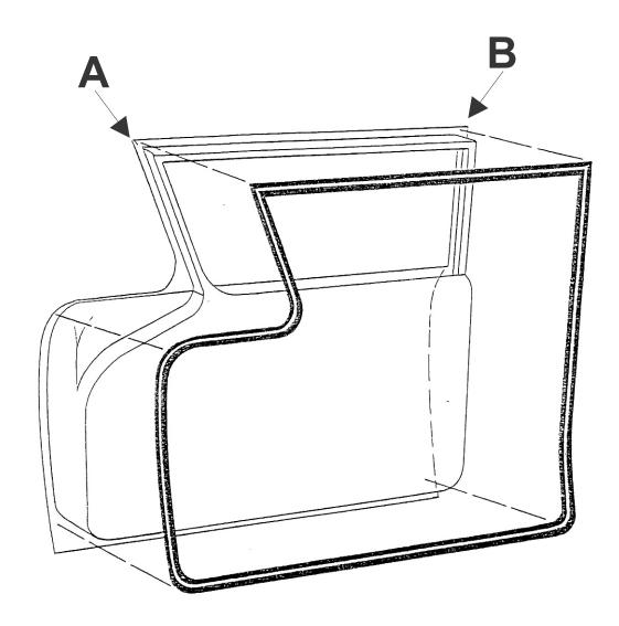
STEP 1: Place the new door seal in position as shown in the above drawing.
